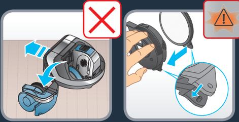
NOTE: If the filter is not correctly fitted in the cap, the error can be also displayed. Please check the good position of the filter.
