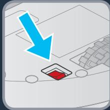
**EN** Turn the robot upside down and turn the power switch ON (I)
