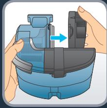
**EN** Twist the black top as indicated with the
