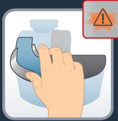
**EN** Remove the dust container by lifting it upwards. The
